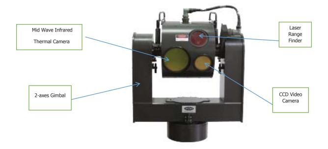
Figure 1. System Sensor Head
