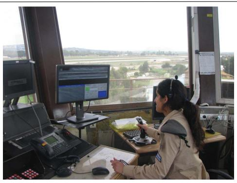
Figure 4. Control and display unit of the SENTINEL system in the ATC tower.
