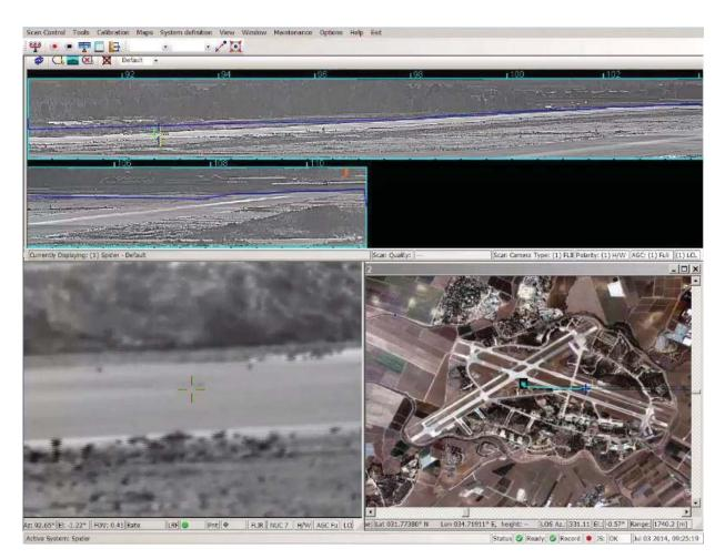
Figure 6. Capture of the SENTINEL display. Zoomed view of the FOD test target shown in Figure 2.1 to confirm the detected foreign object. The system was unable to identify the target at that range.
