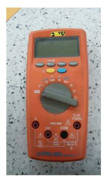
Figure 5. A calibrated APPA 90 Series II Multimeter was used to measure the target object and tarmac temperatures
